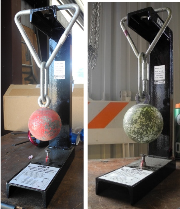
(f) Six new weights (4 kg & 12 lb) were legal but showed a different design or quality problem: They are notably shorter than they legally could be. In spite of that, one of these weights was thrown for a world record. An inspector would do well to inform the owner of this condition:
