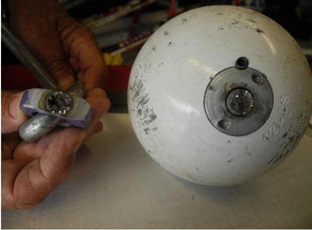
(e) The eye bolt on this new weight snapped during warm-ups on its first trip to the field. While this particular case was probably not foreseeable, it is reasonable to check the eye bolts during inspection for cracks:
