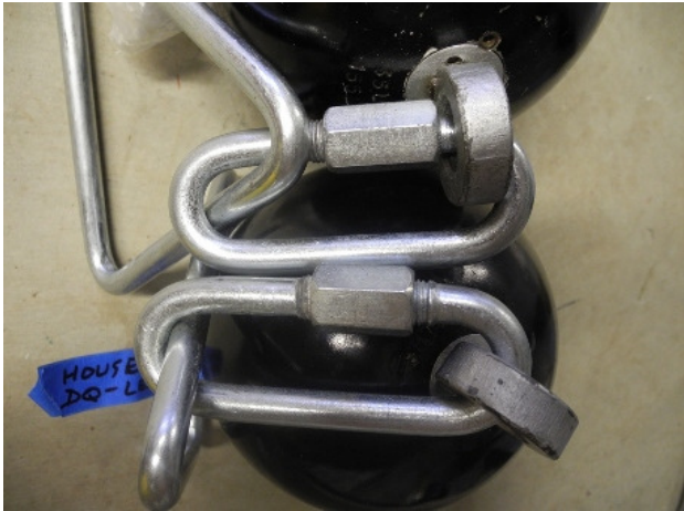
(d) The upper 35 lb weight is of legal length. The lower weight is identical, except its detachable link is longer, making the implement over the legal limit. A third 35 lb weight had the same problem:
